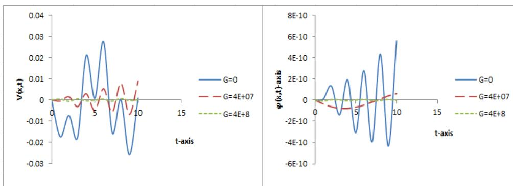
Fig. 3. Transverse displacement & Rotation of the non-uniformly prestressed thick beam under distributed moving load travelling at varying velocity for various values of foundation modulus  $G$  and fixed values of  $N(40000)$  and  $K(40000)$  that traversed by moving distributed force.
