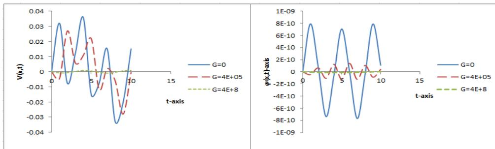
Fig. 6. Transverse displacement & Rotation of the non-uniformly prestressed thick beam under distributed moving load travelling at varying velocity for various values of foundation modulus  $G$  and fixed values of  $N(40000)$  and  $K(40000)$  that traversed by moving distributed mass.
