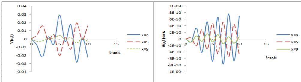
Fig. 7. Transverse displacement & Rotation of the non-uniformly prestressed thick beam under distributed moving load travelling at varying velocity for various values of  $X$  and fixed values of  $N(40000)$ ,  $K(40000)$  and  $G(77000)$  that traversed by moving distributed force.
