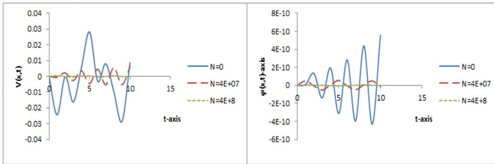
Fig. 1. Transverse displacement & Rotation of the non-uniformly prestressed thick beam under distributed moving load travelling at varying velocity for various values of axial force  $N$  and for fixed values of  $G(77000)$  and  $K(40000)$  and traversed by moving distributed force.
