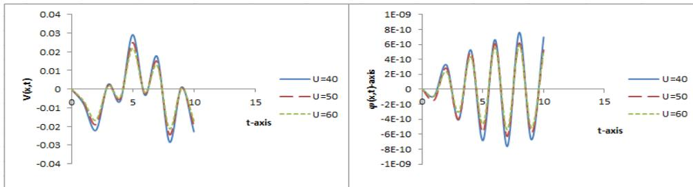
Fig. 8. Transverse displacement & Rotation of the non-uniformly prestressed thick beam under distributed moving load travelling at varying velocity for various values of  $U$  and fixed values of  $N(40000)$ ,  $K(40000)$  and  $G(77000)$  that traversed by moving distributed force.
