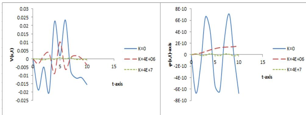
Fig. 2. Transverse displacement & Rotation of the non-uniformly prestressed thick beam under distributed moving load travelling at varying velocity for various values of foundation stiffness  $K$  and fixed values of  $G(77000)$  and  $N(40000)$  that traversed by moving distributed force.
