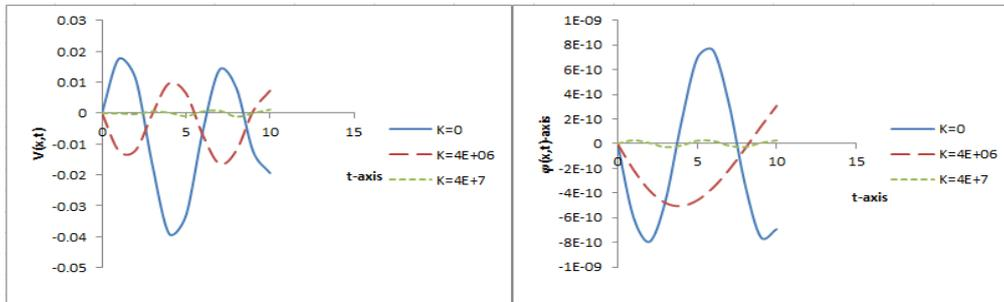
Fig. 5. Transverse displacement & Rotation of the non-uniformly prestressed thick beam under distributed moving load travelling at varying velocity for various values of foundation stiffness  $K$  and fixed values of  $G(77000)$  and  $N(40000)$  that traversed by moving distributed mass.
