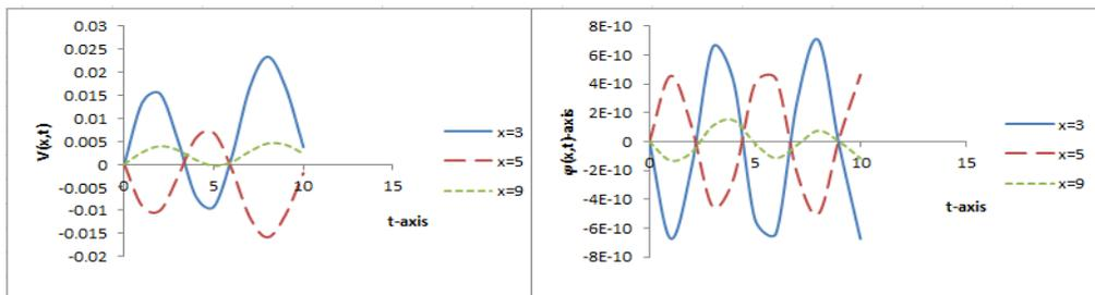
Fig. 9. Transverse displacement & Rotation of the non-uniformly prestressed thick beam under distributed moving load travelling at varying velocity for various values of  $X$  and fixed values of  $N(40000)$ ,  $K(40000)$  and  $G(77000)$  that traversed by moving distributed mass.
