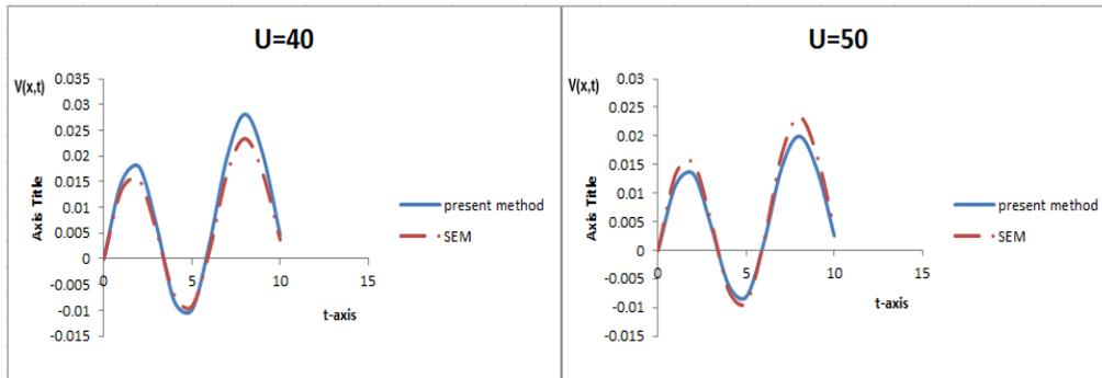
Fig. 12. Comparison of the present method and SEM method  $U=40$  &  $U=50$  of the non-uniformly prestressed thick beam under distributed moving load travelling at varying velocity for fixed values of  $N(40000)$ ,  $K(40000)$  and  $G(77000)$ .
