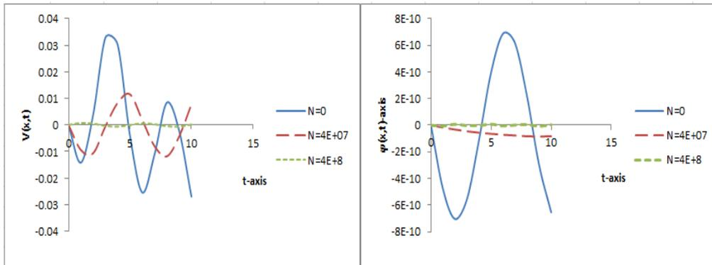
Fig. 4. Transverse displacement & Rotation of the non-uniformly prestressed thick beam under distributed moving load travelling at varying velocity for various values of axial force  $N$  and for fixed values of  $G(77000)$  and  $K(40000)$  and traversed by moving distributed mass.
