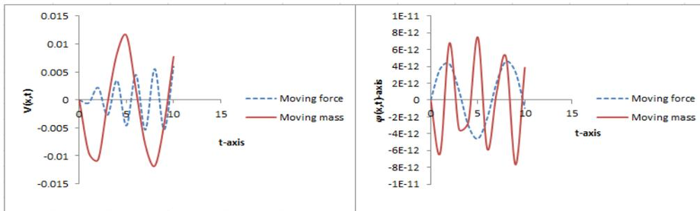
Fig. 11. Comparison of the moving force and moving mass cases of Transverse displacement & Rotation of the non-uniformly prestressed thick beam under distributed moving load travelling at varying velocity for fixed values of  $N(40000)$ ,  $K(40000)$  and  $G(77000)$ .
