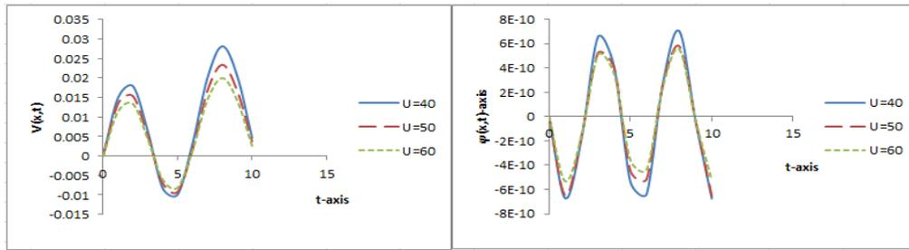
Fig. 10. Transverse displacement & Rotation of the non-uniformly prestressed thick beam under distributed moving load travelling at varying velocity for various values of  $U$  and fixed values of  $N(40000)$ ,  $K(40000)$  and  $G(77000)$  that traversed by moving distributed mass.
